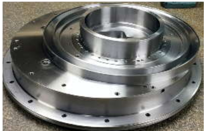
Complete milling of castings for gun drilling machine. Checking for accuracy before moving to Devlieg for boring.
