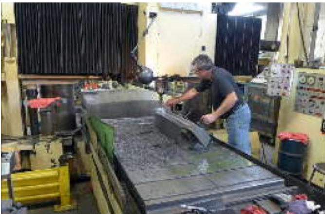
Complete milling of castings for gun drilling machine. Checking for accuracy before moving to Devlieg for boring.
