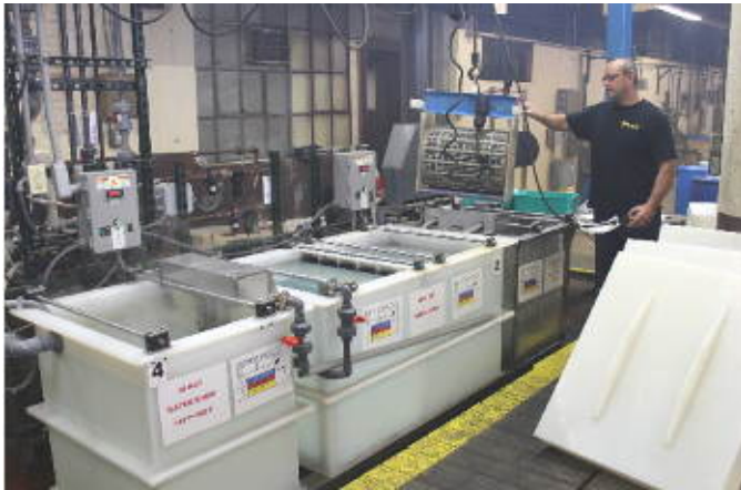
Wilfredo Cancel, Supervisor, processes medical components in this UniMetal Nadcap Certified for both the Citric and Nitric passivation process lines.
