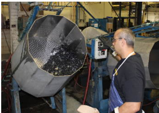
There are 30 of these oblique tumble clean barrels in various sizes. Used with water produces a hand buffed appearance and can work well even on more delicate parts.
