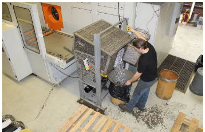
When the customer's parts exit the Roll cleaning machine they are super clean. The parts are re-loaded back into the customer's container which is lined with a plastic bag to maintain part cleanliness.
