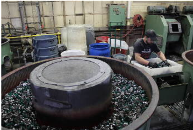
A large vibration tumbler and the operator separating customer parts from the media. Just one of several choices of how to produce the best parts possible.
