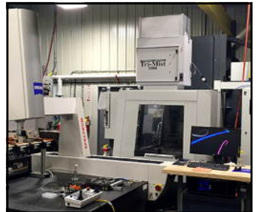
Tri-Mist 1000 mounted on a Haas with the Low Profile Machine Mount and optional 6th stage HEPA Post Filter.
