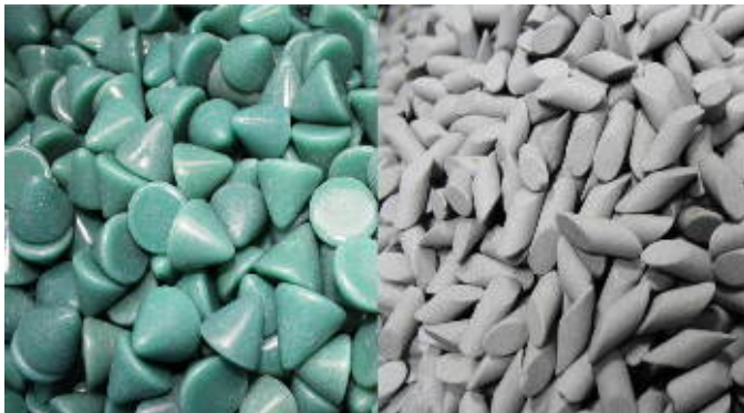
Using the correct media is what tumble deburring and polishing are all about. With advantages in wet or dry processing surface finishes are very predictable.
