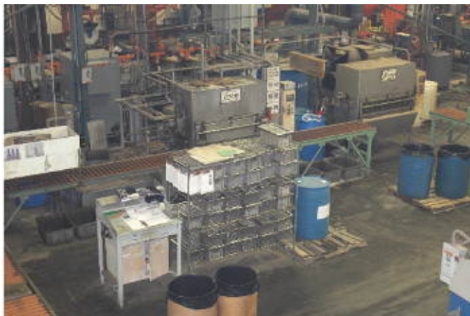
This passivation equipment utilizes stainless steel locked cover baskets. It handles medium to delicate parts that are cleaned, passivated and dried in the baskets.
