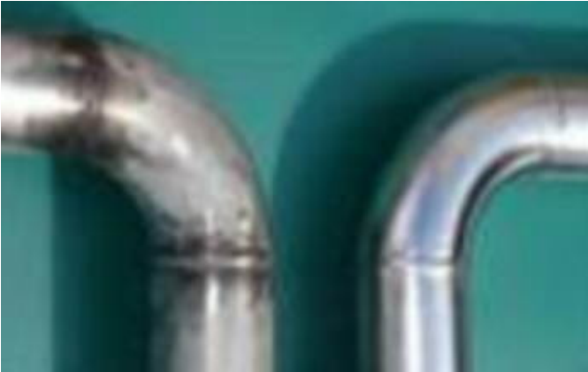
(left) SST welded joint before electropolish. (right) After electropolish, clean and improved.
