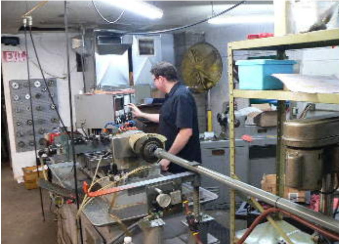
Dan, a graduate of the Seacoast School of Technology school runs an Accuslide Gang Tool CNC for economical, smaller quantity orders requiring close tolerances.
