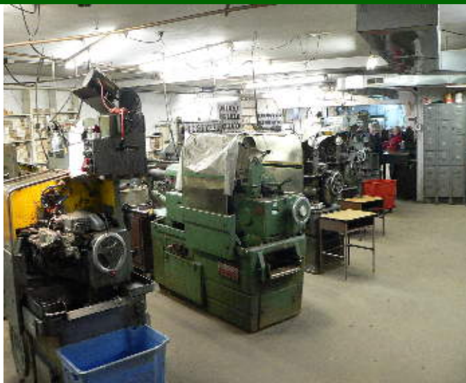
Browne & Sharp single spindle machines are maintained and produce parts to +/- .001" tolerances. Tighter tolerance requirements are set onto bar fed CNC turning centers like the one shown below.
