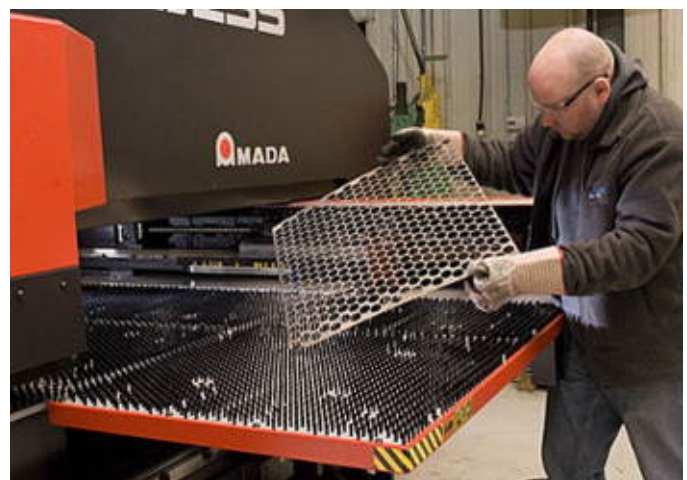
This Amada Turret Press is excellent for larger volume applications and even allows them to produce blanks for hydroforming with minimal waste.
