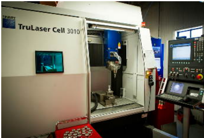
This Trumpf TruLaser, 5 axis laser is the perfect machine to trim parts to perfection following the hydroforming.
