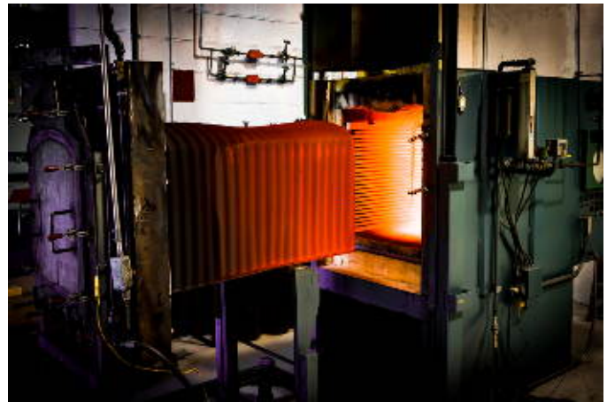
This hydrogen atmospheric controlled heat treating furnace is used to anneal finished or semi formed parts, removing the work hardening that occurs when metal is transformed. MuShield has two of these hydrogen heat treating furnaces to heat treat components up to 2100F.
