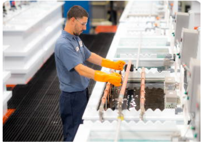
Electropolisher loads a rack of parts into an Electropolishing tank. All jobs that are processed at NEE have documented work instructions listing all key processing and inspection variables.
