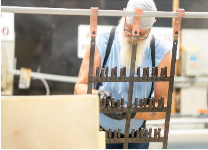
This worker performs a very important process of loading the parts onto electrical conductive racks. The connection has to be secure and not interfere with critical surfaces being treated.
