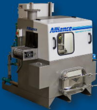
Aquamaster CB-1200E Conveyorized Belt Cleaning System
