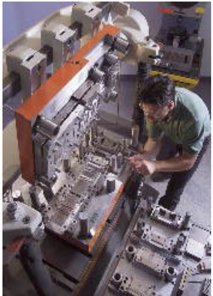
A tool & die maker assembles a progressive die.
