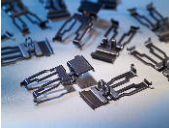
Spring legs can be formed in the press with cam operated in-die slides.
