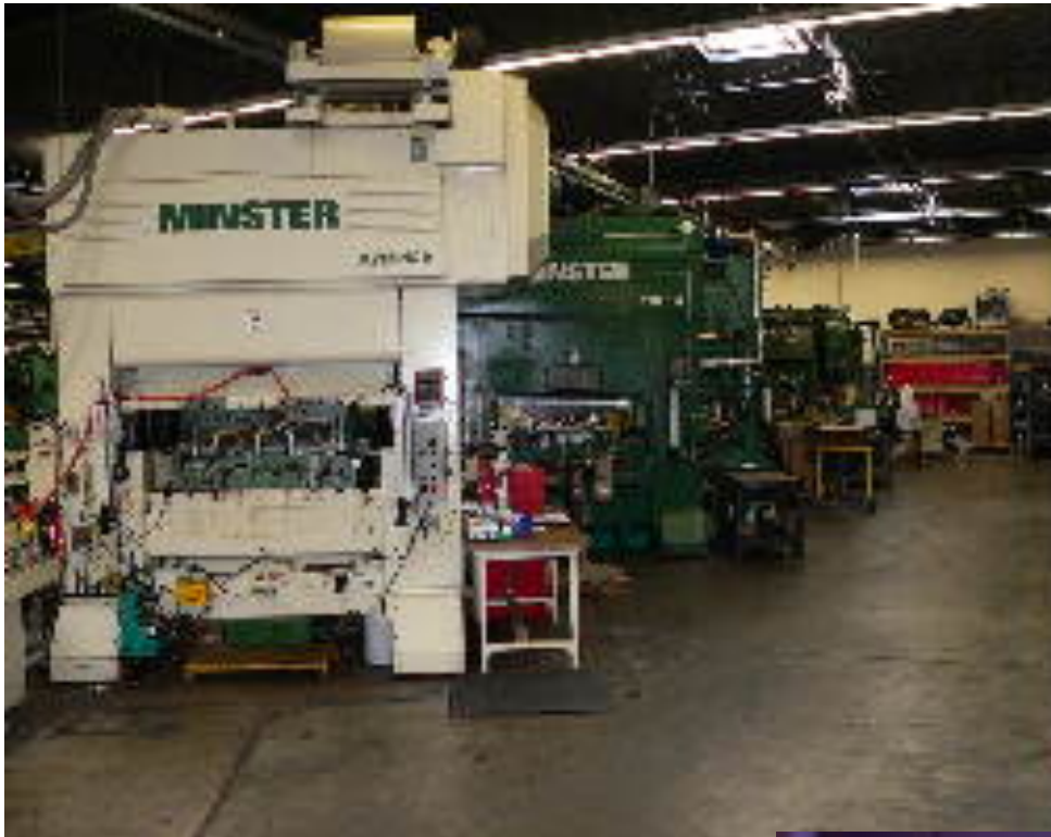
(Above) Once the tools are made in their 30 man tool & die shop, Hobson Motzer has state-of-the-art presses to stamp parts, like this 180 ton Minster press. They have 26 presses ranging from 30 to 180 tons.
