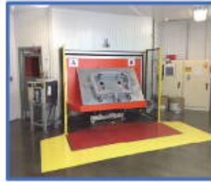
Robotic Laser Deletion System For Automotive Windshields
