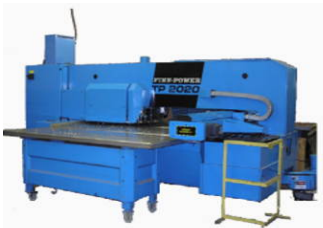
(L) The Finn Power TP2020 is a 33 ton high speed punch press. (R) The operator sets up the punches and dies before running the pile of sheet through the press.
