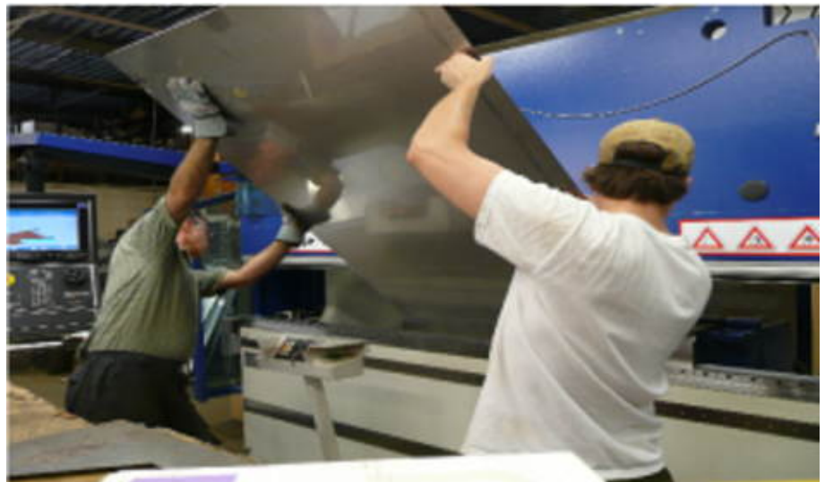
Shearing, folding and bending operations are vitally important at Howard Products. It takes two people to hold this thick sheet of Aluminum plate up for folding. Accuracy is not vital, Continued on page 7
