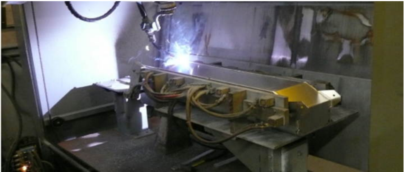
Robotic welder takes the labor out of longer repetitive jobs and produces a smoother flow for great welds.
