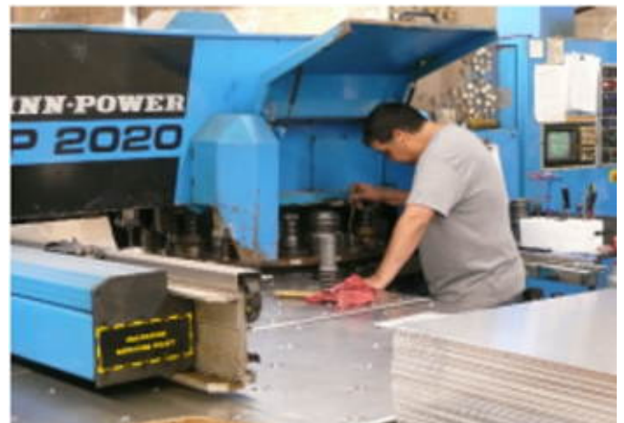
(L) The Finn Power TP2020 is a 33 ton high speed punch press. (R) The operator sets up the punches and dies before running the pile of sheet through the press.
