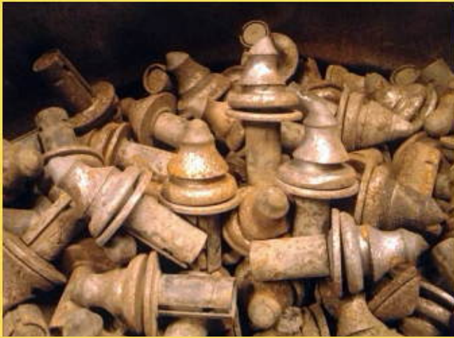
Tungsten Carbide milling bits used in asphalt road grinding operation.
