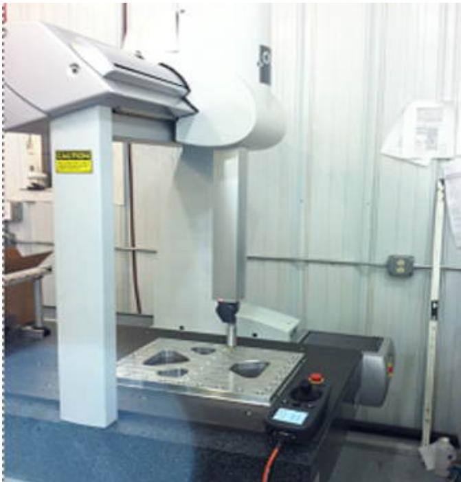
Brown & Sharpe Global Performance CMM (Coordinate Measuring Machine) is just a slight indication of Kokos emphasis on quality.
