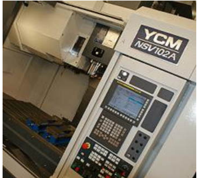
Haas, YCM and Bridgeport Milling machines with up to 64" x 32" x 30", 5 axis and 24 tool changers.
