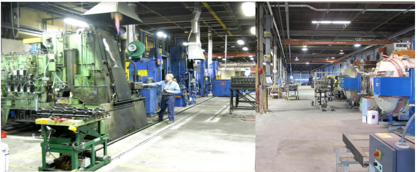
An impressive line of carburizing furnaces fill the left wall of the shop, while the right side wall is a wall of state-of-the-art vacuum furnaces.
