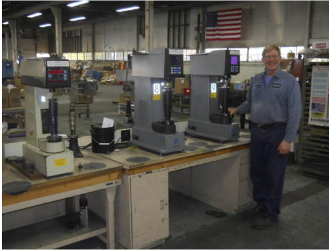
Making sure hardness of parts is in conformance to customer requirements is just one area of metallography and micro hardness testing that they perform.
