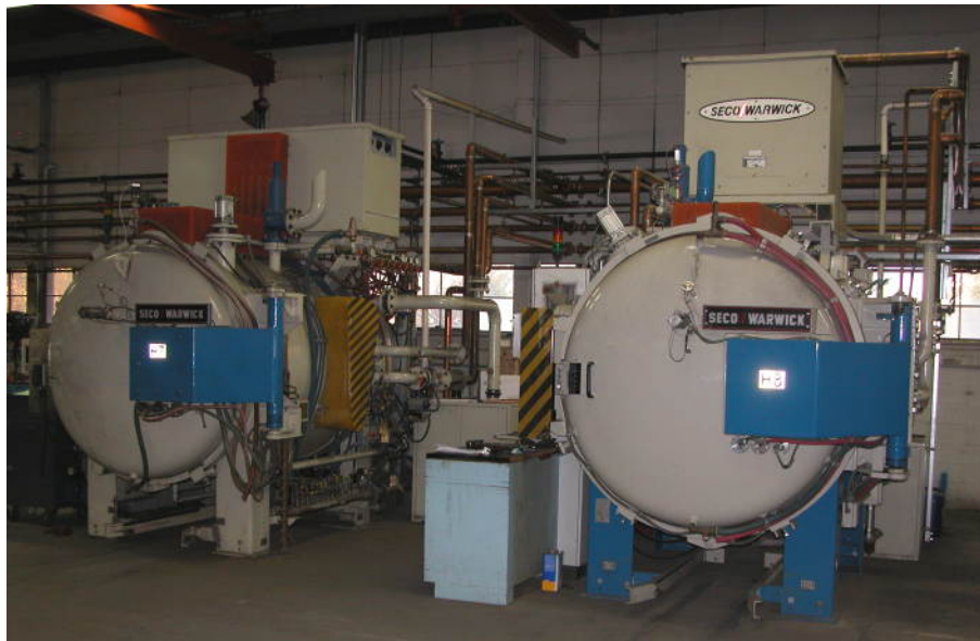
The right hand vacuum furnace is the newest addition to the shop with more and more customers wanting the bright and shiny heat treatment for their needs.
