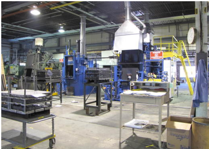
Parts are often racked to reduce distortion during the heat treat process as seen in this staging area.
