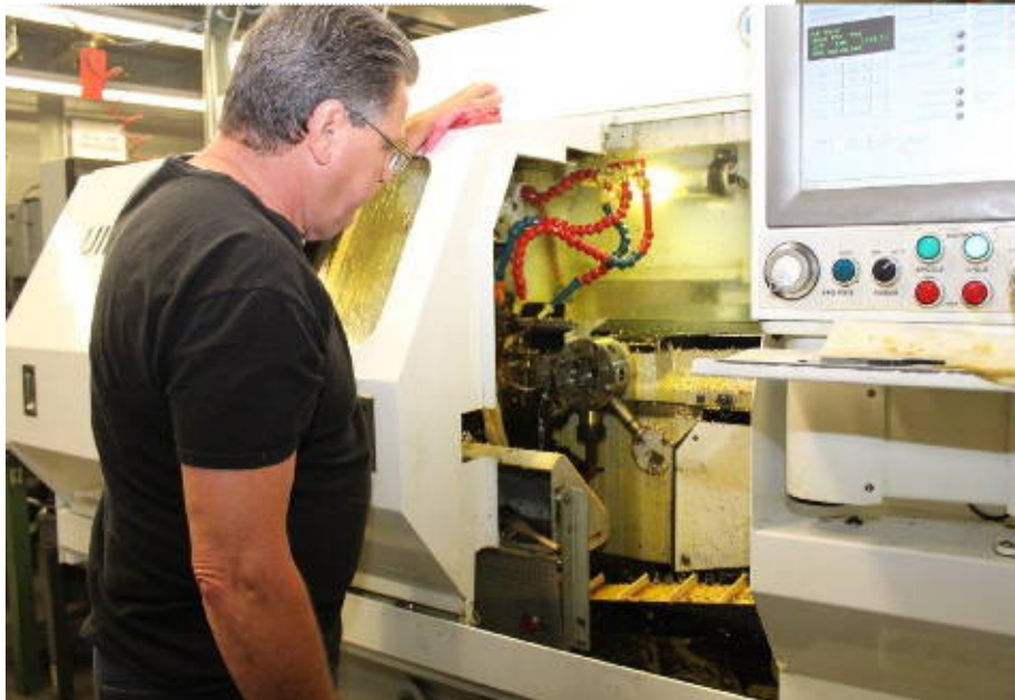
(left) The machine pictured is one of only 20 such machines ever built, combining the speed of Brown & Sharpe screwmachines with the accuracy of modern CNC machines.
