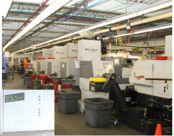
(above) Modern 6- and 7- axis Sliding headstock machines with capacity up to 42mm ( 1.654") diameter.
