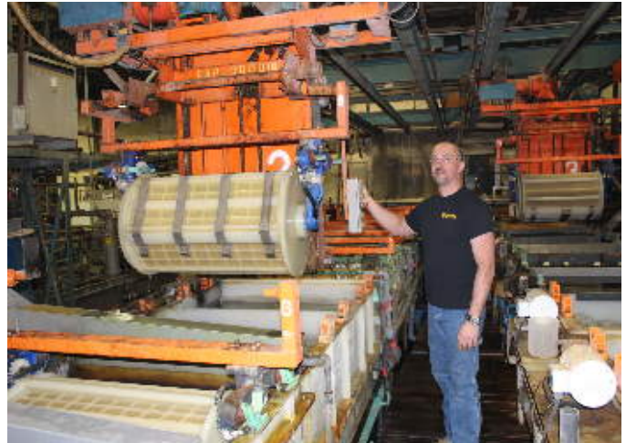
Armand DeAngelis, Plating Supervisor, moving a typical plating cylinder on a large acid zinc automatic plating line. Normal output on this line is 1,000 lbs per hour
