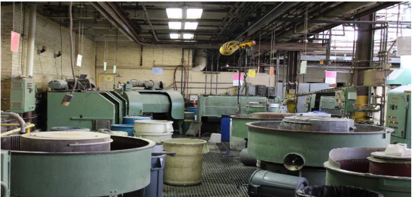
UniMetal's vibratory deburr department. Horizontal rotary and small to large vibratory bowls handle various size parts. Inventory stocks the correct media required to remove burrs on both outside and inside of parts.
