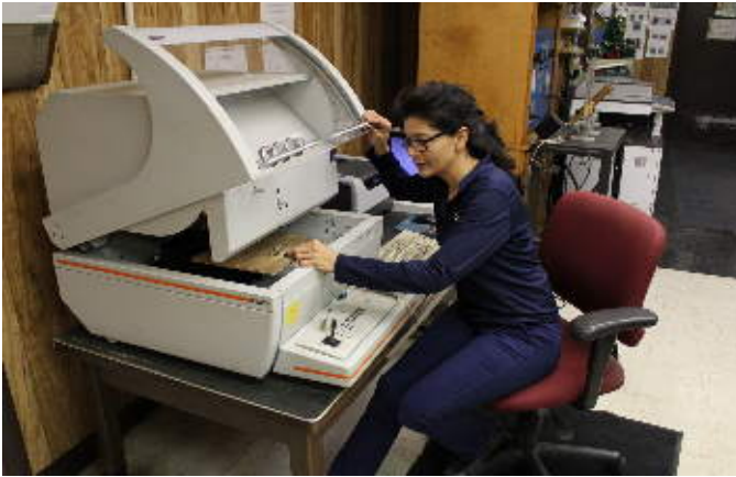
Aida Poventud, Director of Quality is performing a plating thickness measurement. With this X-ray Fluorescence machine she can also identify multiple thickness levels of multiple under coats such as gold and nickel over a copper flash base.
