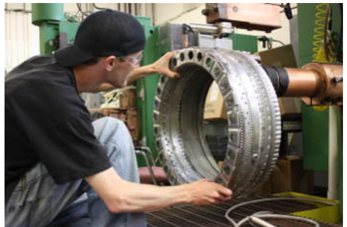
Resistance spot welding of a combustion liner.
