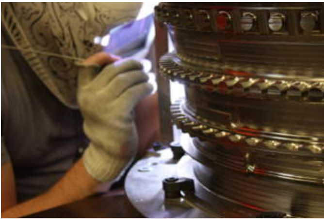
GTAW welding (Gas Tungsten Arc Welding) of a jet engine case assembly.
