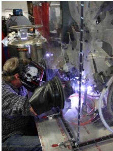
Resistance welding in inert gas chamber.
