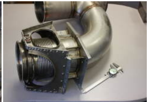
Duct assembly that was resistance and fusion welded.
