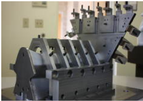
5 Axis machining fixture designed and built by Lynn Welding.
