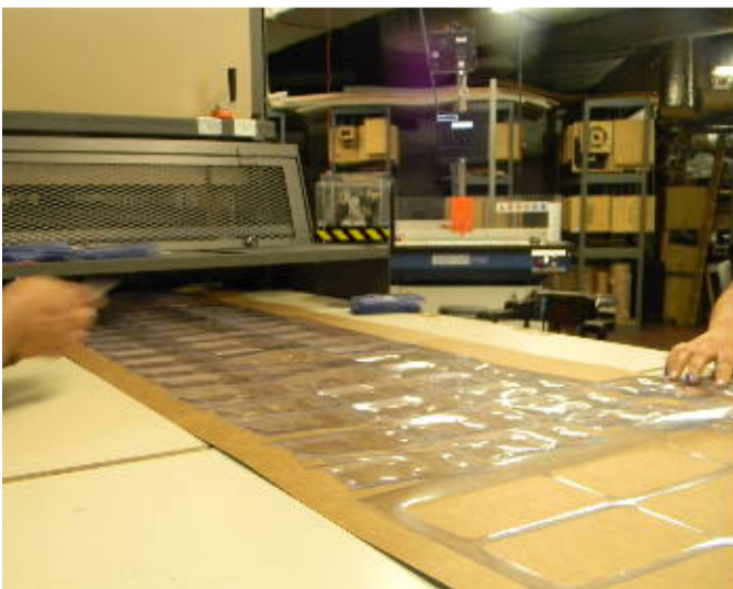
45 ton Tarp press containing a multi position die providing high speed efficiency and low cost. CRT cutting PVC for an electronics packaging application.
