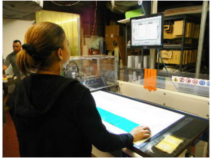
Uploading a customer drawing which will then be precisely cut all without the expense of tooling.
