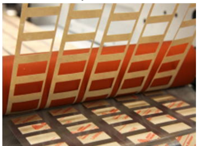
High speed kiss cut tape allows for easy product assembly. Cutting tape, adhesives and pads are one of CRT's specialties.
