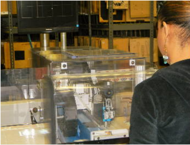
Die-Less knife cutting offers a clean and tight tolerance alternative to die cutting.
