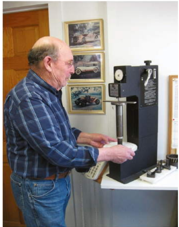
Harold Snow, Snow's Heat Treatment measures hardness to verify he is meeting the purchase order requested specification.
