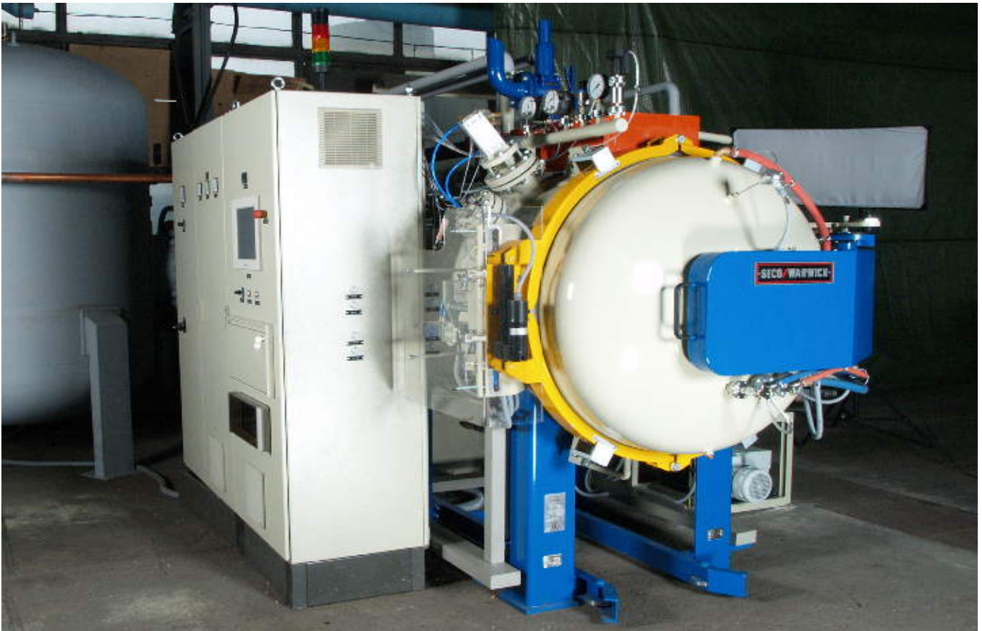
Horizontal vacuum furnace with high-pressure quench and low pressure vacuum carburizing; Hot zone: 24"/600mm x 18"/450mm x 24"/600 mm; Hearth rating: 400 pounds/180 kg. Photo courtesy of SECO/WARWICK"
