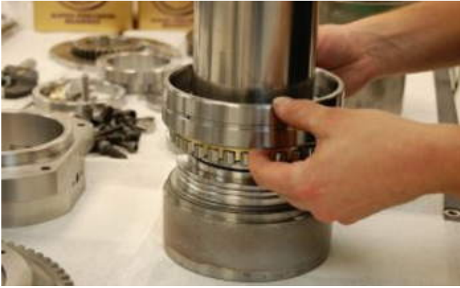
When re-assembling the spindle, our technician checks the preload on the tapered bearings to insure proper performance in your spindle.
