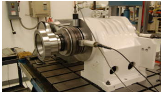
Every spindle must pass through a break-in before final high speed run up. Numerous tests are performed to verify the spindle meets and is in an as new condition.
