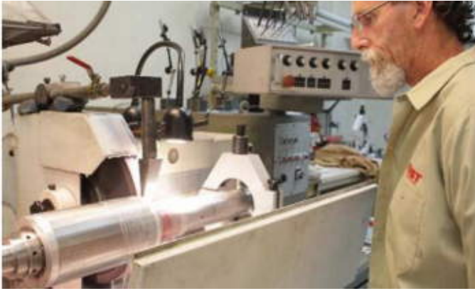
Grinding bearing journals to micron tolerances takes a highly skilled technician and the right equipment. This is done at High Speed Technologies every day.
