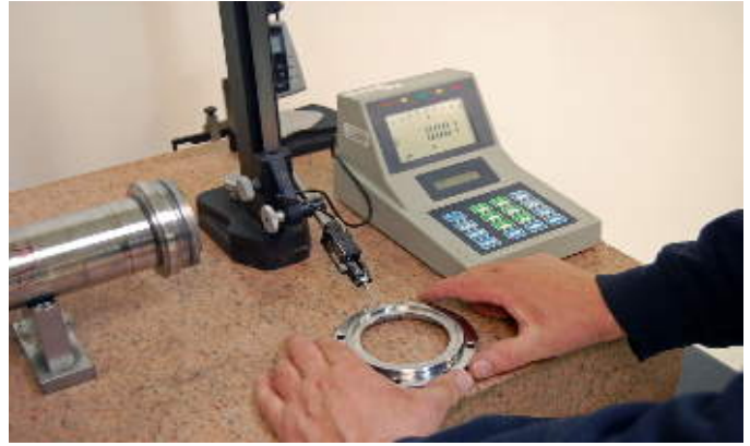
Spacer sets between bearings must be ground in matched sets to precise micron measurements.
