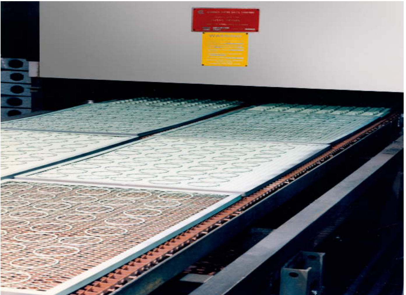
Conveyor line ovens are utilized to cure the coating.
