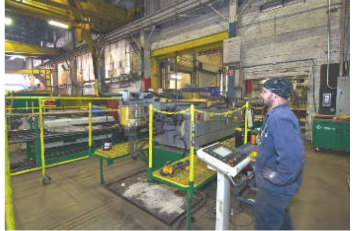
UMS technician uses a computerized bending machine to complete a customized pipe project.
