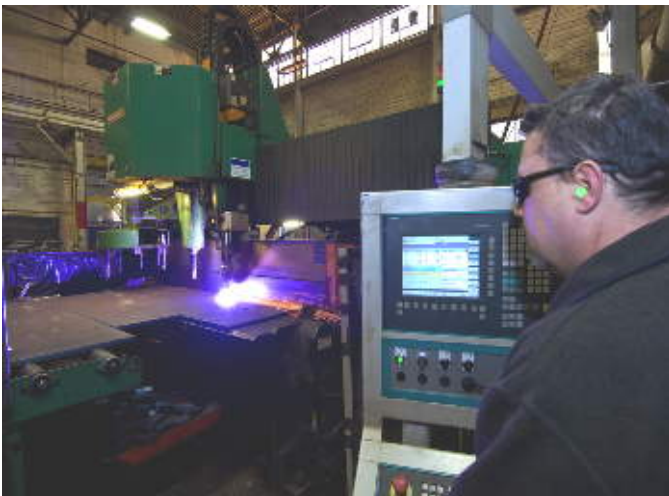
UMS tradesman operates a high-speed plasma/oxy machine, which is capable of drilling, milling, tapping and doing countersunk holes from ¼”-3” material.
