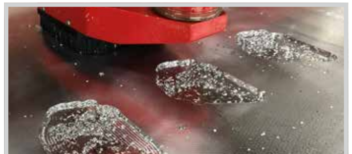
CNC milling pockets in aluminum with large vacuum table
