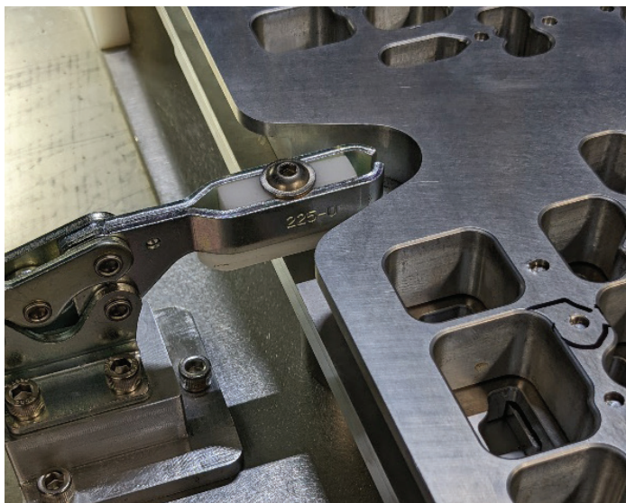
Figure 3 shows a typical lever clamp to fix the pallet fixture in place, where the pallet fixture was pre-loaded with components and assembled externally.
