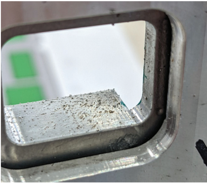
Figure 4 shows an image of a window and the resulting ejected materials. This view is from the laser side.
