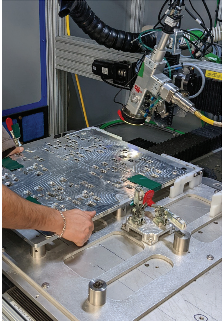
Figure 2 shows a palletized fixture being placed into the laser welding tool.
